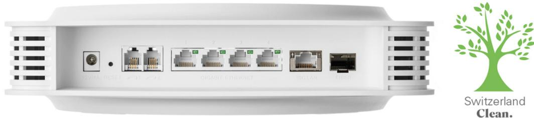
*Salt's Fiber Box comes with four Ethernet 1 GB ports, one Ethernet 10 GB port, two telephony ports as well as 2 USB 3.0 ports (not visible on the above picture).*
